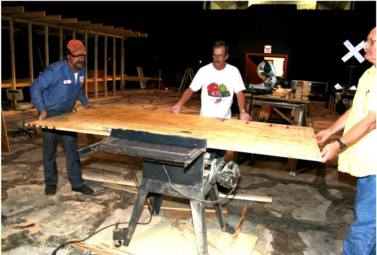
Tracy Ball, Earl Carrel and Virgil Doyle ripping panels for staging yard tracks
