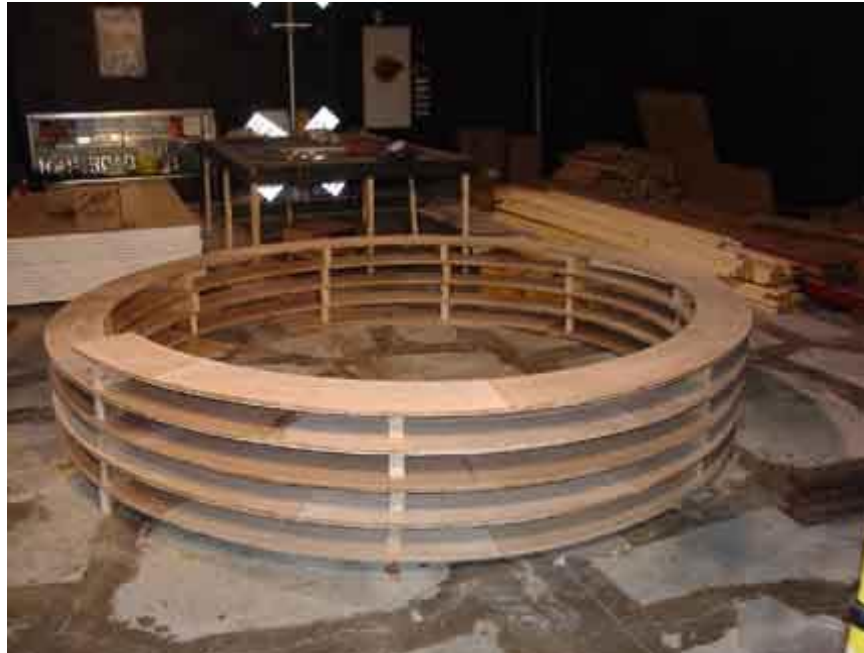
The ARM helix (A.K.A. The Wooden Slinky ). Shown with blocks between layers before holes for the supporting rods have been drilled.
