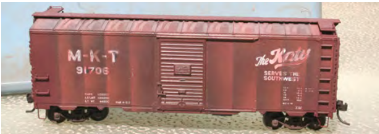
A 1944 Modified '37 Boxcar with 4/4 Improved Dreadnaught ends, a diagonal panel roof and an inside height of 10'4"
