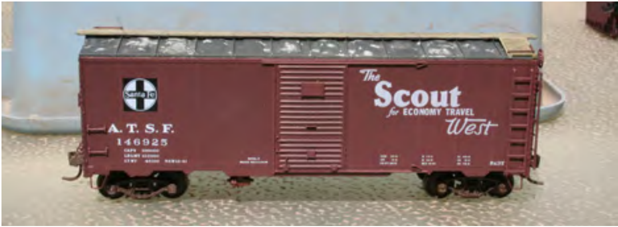
A 1941 Modified '37 boxcar with a raised panel roof, 5/5 Dreadnaught ends and a 10'4" inside height.
