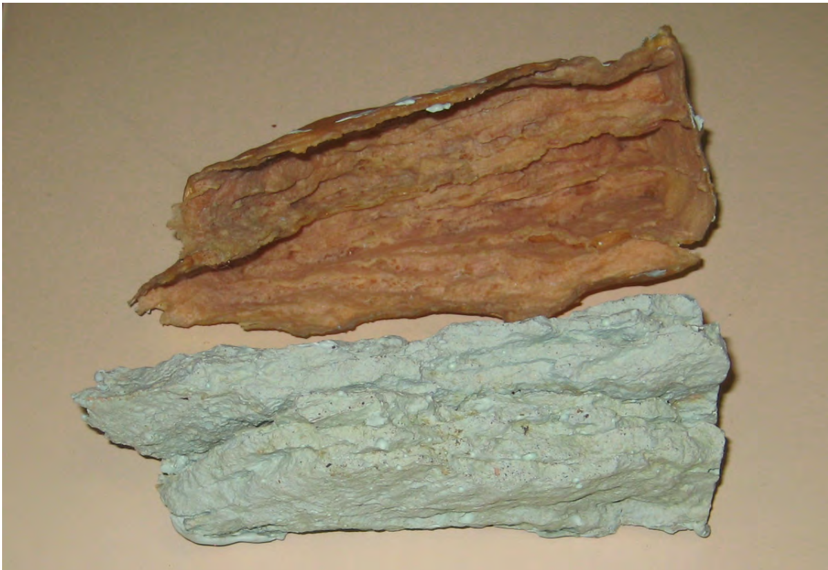
A flexible latex mold (top) and a Bondo hollow casting (bottom). The Bondo casting is much lighter than a Hydrocal casting. Bondo decorates similarly to Hydrocal.
