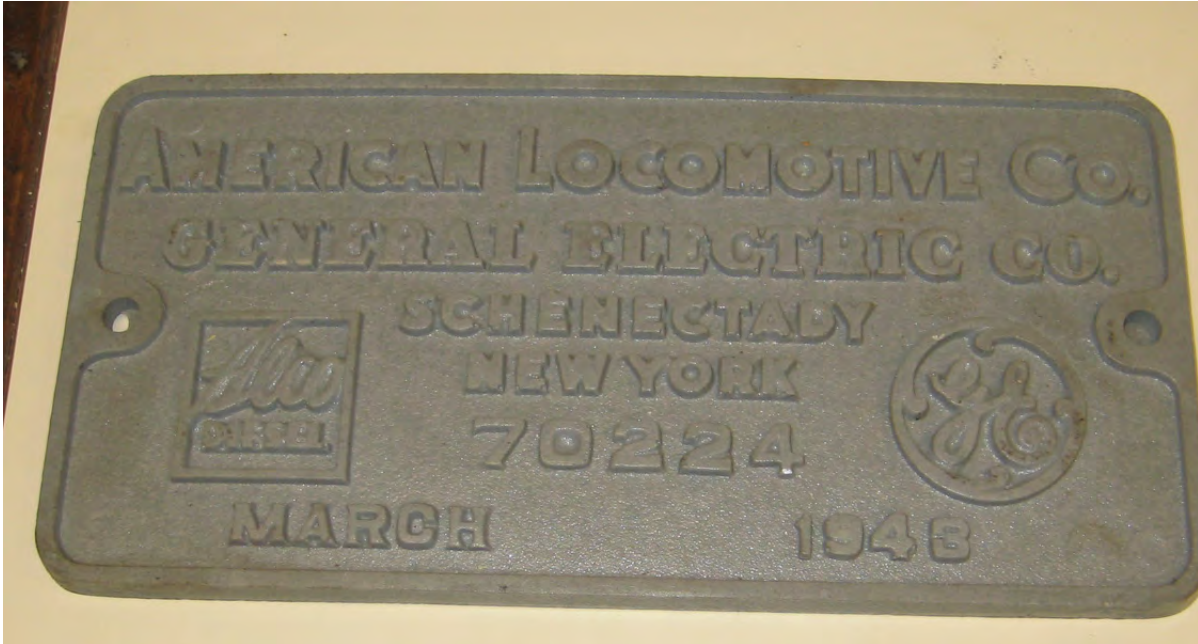
A resin replica of the builder's plate from our Alco-GE S-2. The mold was RTV rubber and its size is 6 inches x 11 7/8 inches.
