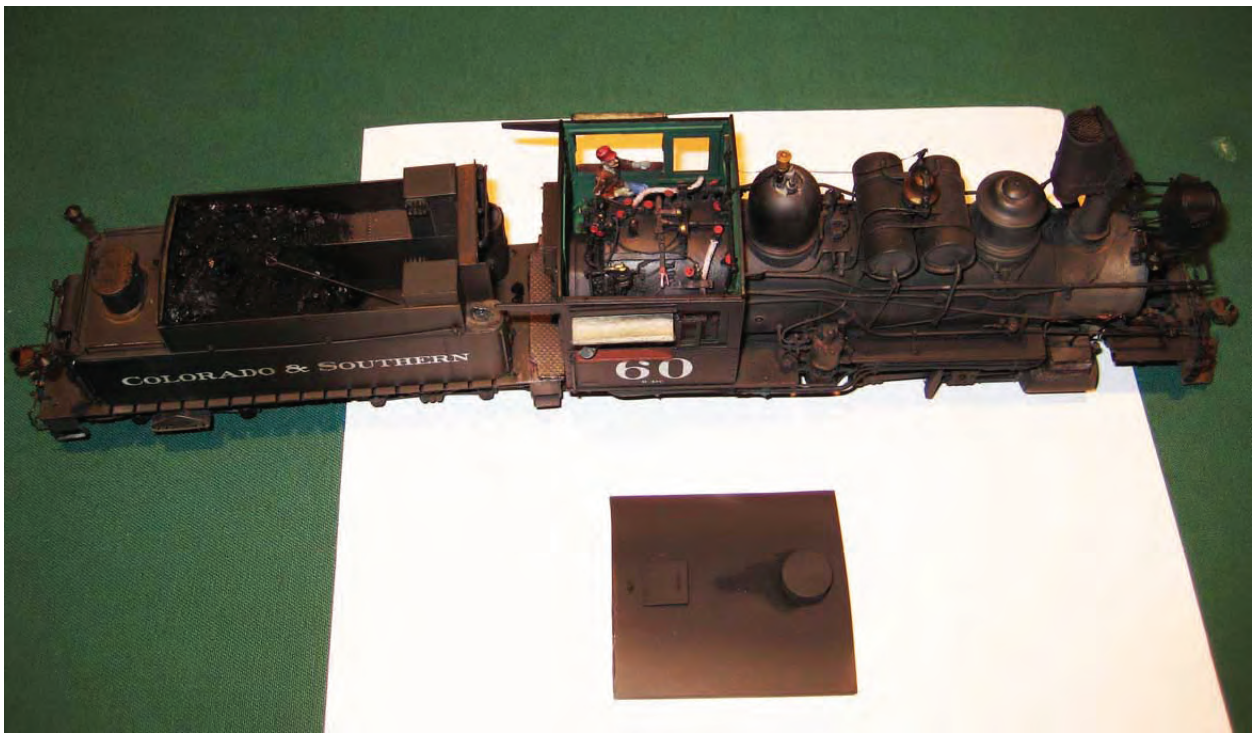
Colorado & Southern #60, with a fully-detailed cab interior and characteristic C&S Bear-trap that accumulated cinders from the exhaust.
