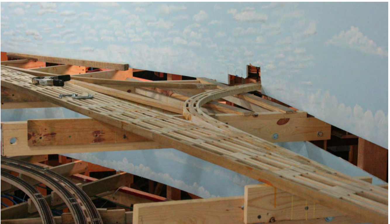
HO Scale Layout: West leg of Lubbock Junction wye in Canyon on the upper level of the layout.
