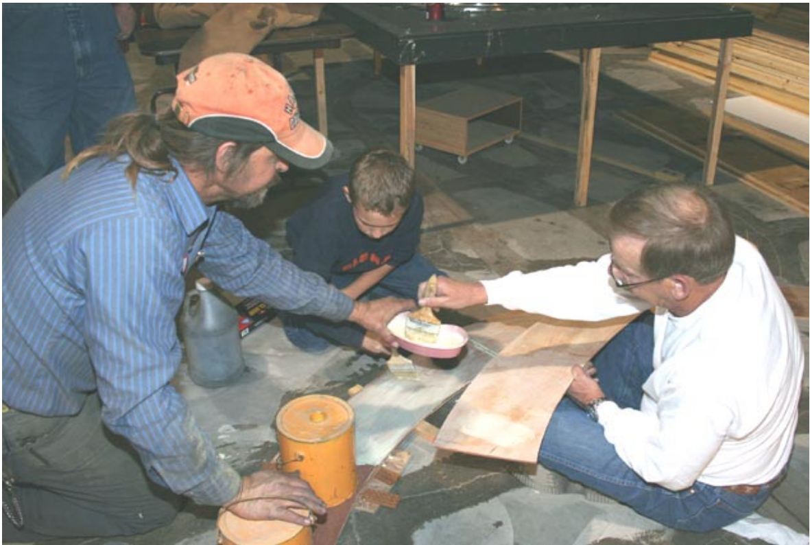
Tracy holds the glue while Earl brushes in onto panel. Austin spreads glue on bottom layer.
