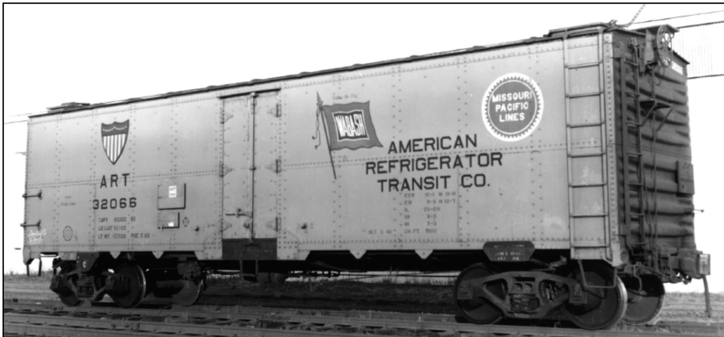
ART 32066 from series 32000-32999, renumbered from original series 24100-24199, built November 1940 by ART from kits furnished by American Car & Foundry Co. (lot no. 2094). The car had been repainted at Pueblo, Colorado in May 1960. Note the placard boards had been lowered, an A.A.R. practice begun in 1954. An electric fan was installed below the side sill at the left bolster. Also, the car received yellow side sills and the reporting marks bars and periods had been dropped. Photo circa 1960 or 1961.
