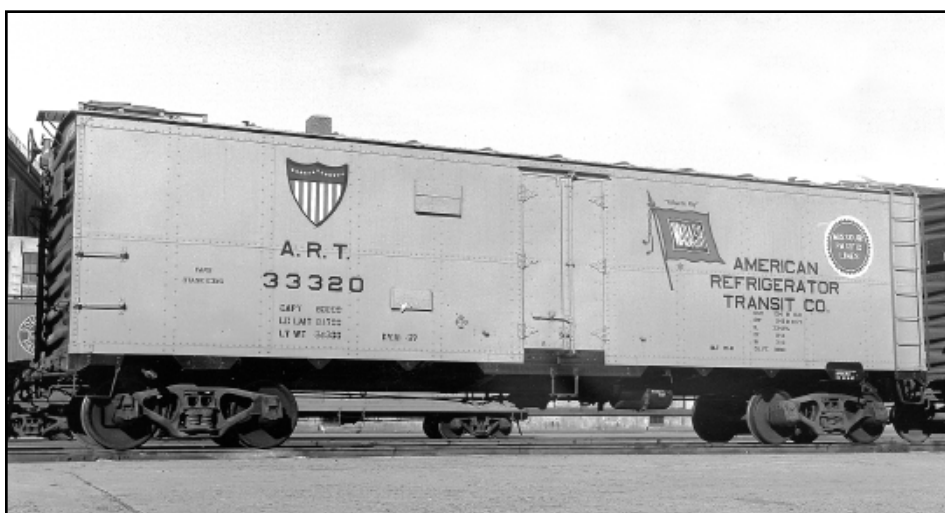
Bottom- ART 33320 from series 33000-33999, renumbered from original series 24200-24349, built October 1941 by ART from kits furnished by American Car & Foundry Co. (lot no. 2266). The car shown was freshly repainted at Kingsville, Texas in November 1957. At that time, the reporting marks bars had been dropped but periods were still being used. Also note the trademark symbol under the Wabash flag that was used after March 11, 1957. The B-end is at the left, suggesting the Wabash flag and MoPac emblem positions had been reversed. The car was equipped with internal Equipco mechanical air-circulating fans. Hatch covers with rounded corners are evident in the photo taken November 30, 1957, at Providence, Rhode Island.
