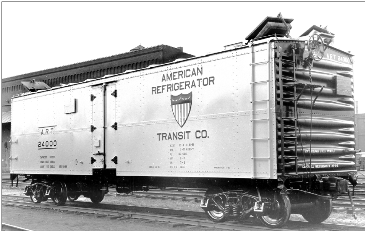
Top Previous Page and Above- ART 24000 from series 24000-24099, built November 1939 by ART from kits furnished by American Car & Foundry Co. (lot no. 1922). Two views of the class car display the A-end and B-end. Close inspection of the photos reveals that the hatch covers were smooth plate steel with square corners. This was the first of 775 nearly identical cars assembled by ART from 1939 through 1946. Note the position of the placard boards on the upper portion of the sides and ends plus the route card board on the door. Sides were painted yellow, ends and roof were painted Inco Red, and underframe, trucks, side sill, rectangle under the door, and door hardware were black. The ART shield was red, white, and blue with black outline. Stencils on the sides were black. Stencils on the ends were white.
