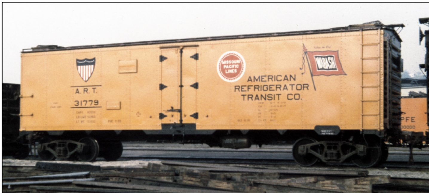
ART 31779 displays the typical paint scheme applied to ART ice reefers during the post-1950 period. In this instance the large Wabash flag was located near the ladder at the A-end of the car. The car was built late 1936 and came from original series 22979 through 23999. Photo is dated January 1956 at an unrecorded location.
