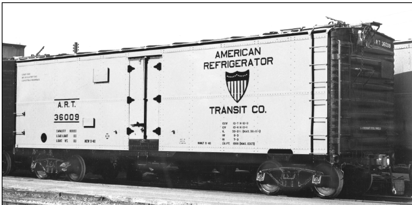
ART 36009 from series 36000-36024, built September 1946 by ART from kits furnished by American Car & Foundry Co. (lot no. 2918). Cars in the series came with Dreadnaught ends with round corners, Preco electric fans, Universal XL power hand brakes, and Apex Tri-Lok running boards. Hatch covers had rounded corners. A note in the ORER states "Cars in the series are operated in special service and should not be handled in the tide movement but handled strictly on record rights and in home routes so they can be returned to assigned points."
