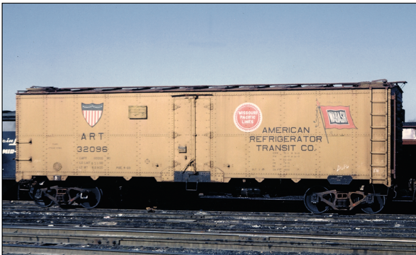
ART 32096 from series 32000-32999, renumbered from original series 24000-24099, built March 1940 by ART from kits furnished by American Car & Foundry Co. (lot no. 1922). The car had been repainted at Pueblo, Colorado in 1960. The placard boards remained in their original high positions and evidence, when compared to the photo of 32066, that the placard applications were not consistent. A Preco electric fan was installed above the side sill at the left bolster. The car received yellow side sills and the reporting marks bars and periods had been dropped. Photo taken ca. 1963, at St. Louis, Missouri.
