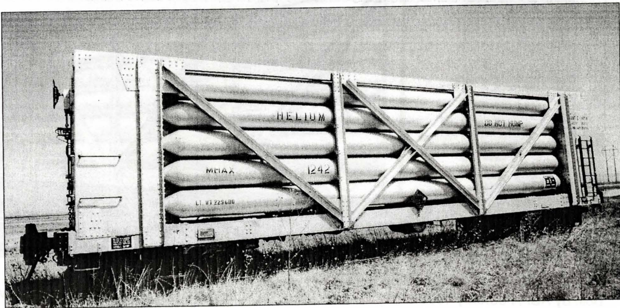
Four-and-One-Half Generation: 30-Tube Car Built by Darby Corporation; September 1958 1020-1025 (Car 1242 is ex. ATMX 1021 shown at Amarillo Railroad Museum in 2001.)
