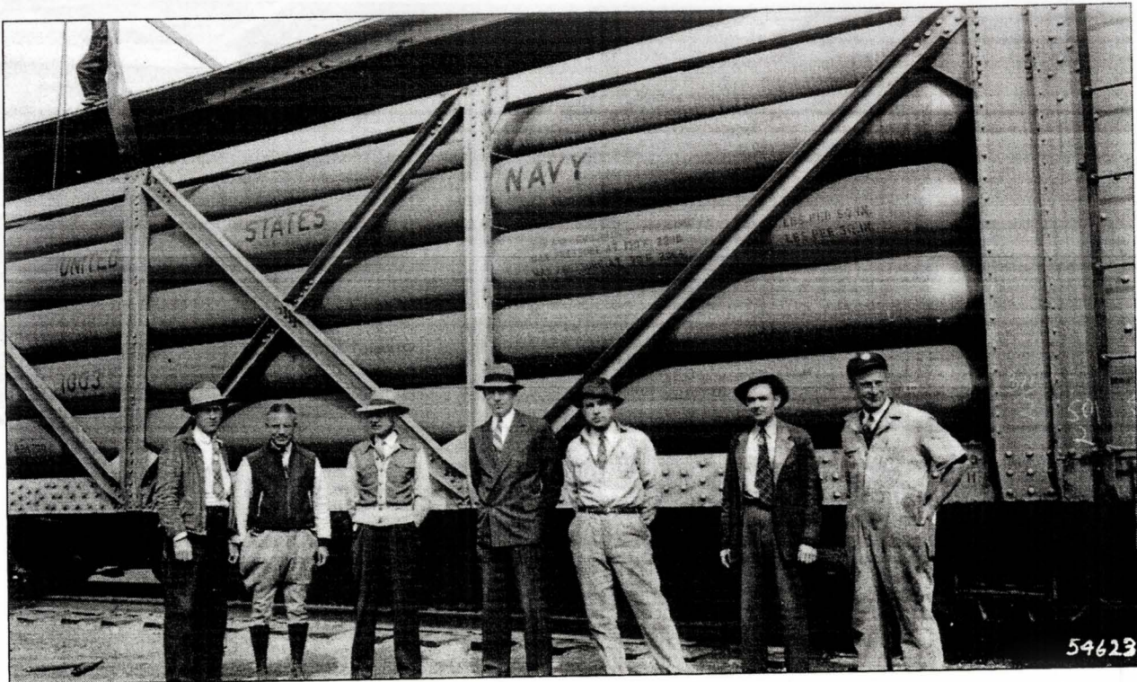
First Generation: 28-Tube and Second Generation: 30-Tube Cars Rebuilt Rebuilt by US Bureau of Mines with 'X' bracing and new 45° bracing ca. 1942. All lettered UNSX. 1002-1012
