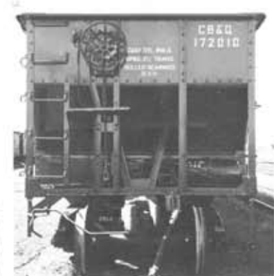
Below, one of the first group of Chinese red cars, HT-10B CB&Q 172010, in a pair of Havelock builder's views dated April 5, 1960. The glossy black-painted roller bearing trucks are all but hidden in shadow.—CB&Q photos, Rod Masterson collection
