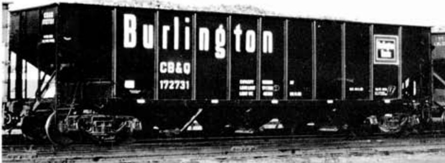
Painted black for coal service but seen here (at Denver in December 1966) loaded with sugar beets, outside-braced rebuild Q 172731 had been turned out of Havelock just a month earlier.—Hol Wagner
