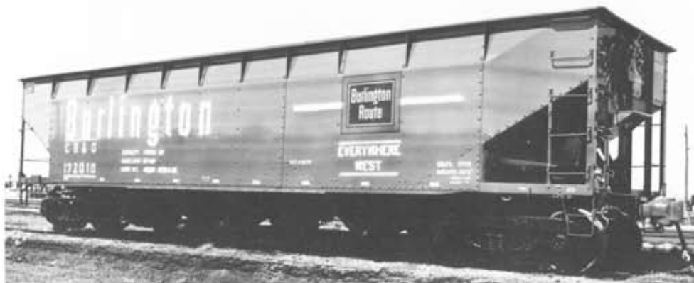
Below, one of the first group of Chinese red cars, HT-10B CB&Q 172010, in a pair of Havelock builder's views dated April 5, 1960. The glossy black-painted roller bearing trucks are all but hidden in shadow.—CB&Q photos, Rod Masterson collection
