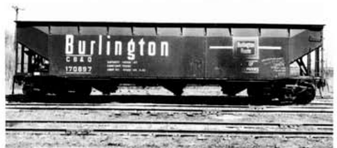
While it looks the same as the 170496, the 170897, here in a right side view at Eola, Illinois, on May 1, 1963, is actually painted black rather than Chinese red, since the triple hoppers were used primarily in coal service. Note the partially obscured "Way of the Zephyrs" slogan.—CB&Q photo, Rod Masterson collection
