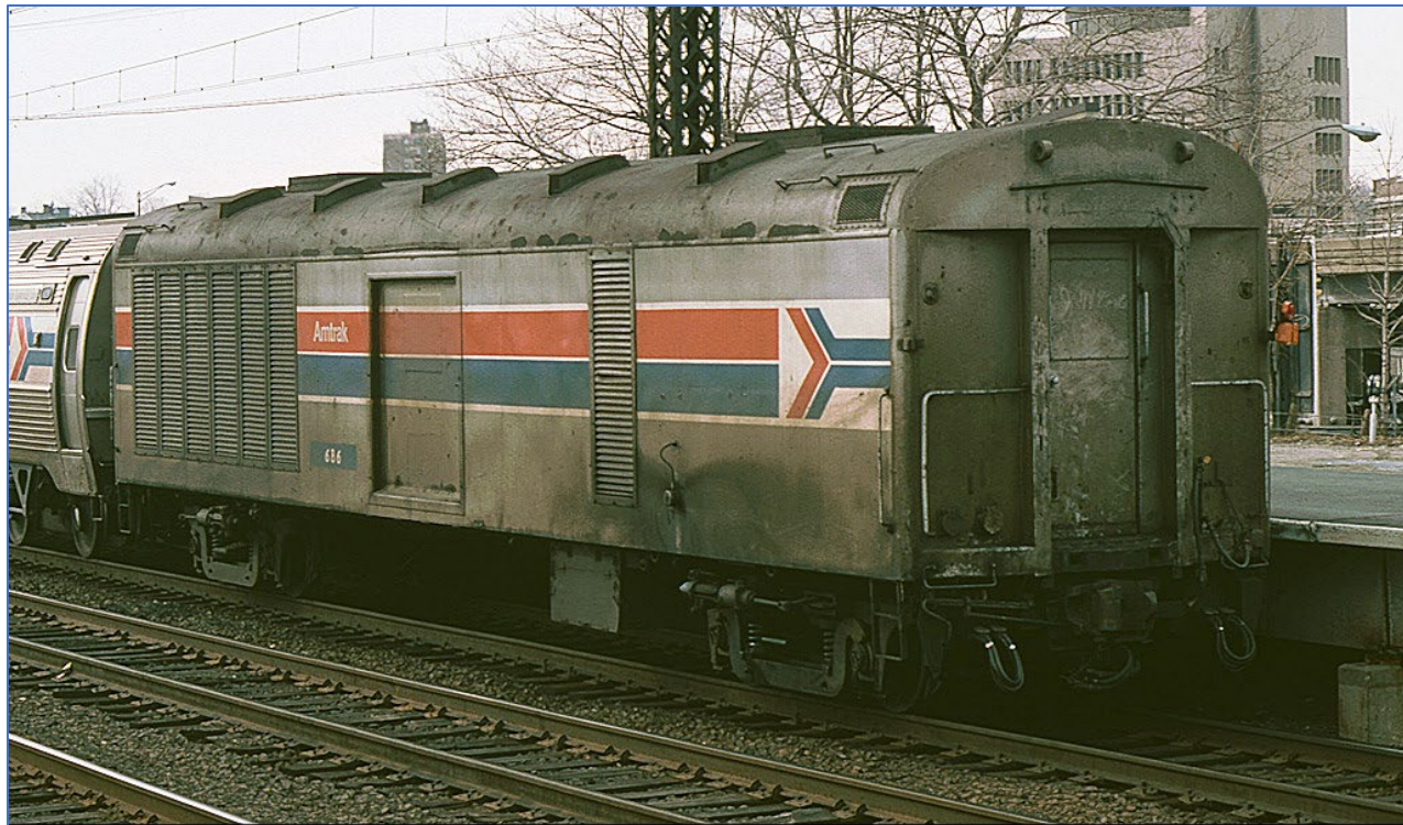
Above. Amtrak 686 (ex-USAX 89625) Below. Amtrak 1293 (ex-USAX 89661) both at Stamford, CT in 1976. Amtrak converted these ex-USAX cars into HEP (Head End Power) cars Both photos Christopher Palmieri Col.
