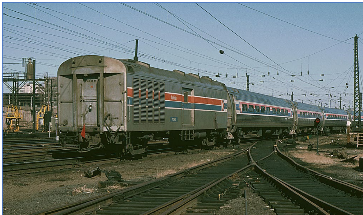
Above. Amtrak 686 (ex-USAX 89625) Below. Amtrak 1293 (ex-USAX 89661) both at Stamford, CT in 1976. Amtrak converted these ex-USAX cars into HEP (Head End Power) cars Both photos Christopher Palmieri Col.
