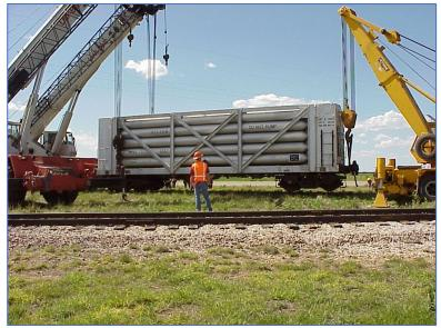
Once the car's brake rigging was detached from the trucks, a yellow Pettibone and two white and red Link-Belt cranes were used to pick the car up off the trucks. The trucks were lifted off the pallet company spur and placed on one of our tracks. Finally, the car body was slowly and carefully moved move over the trucks and lowered into place. Considering that the car weighs 100 tons, the was not an easy task!
