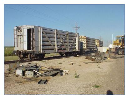
Preservation wasn't to be the fate of most helium transport cars. At the siding of the retired Amarillo U.S. Bureau of Mines plant three helium cars are in various stages of scrapping.
