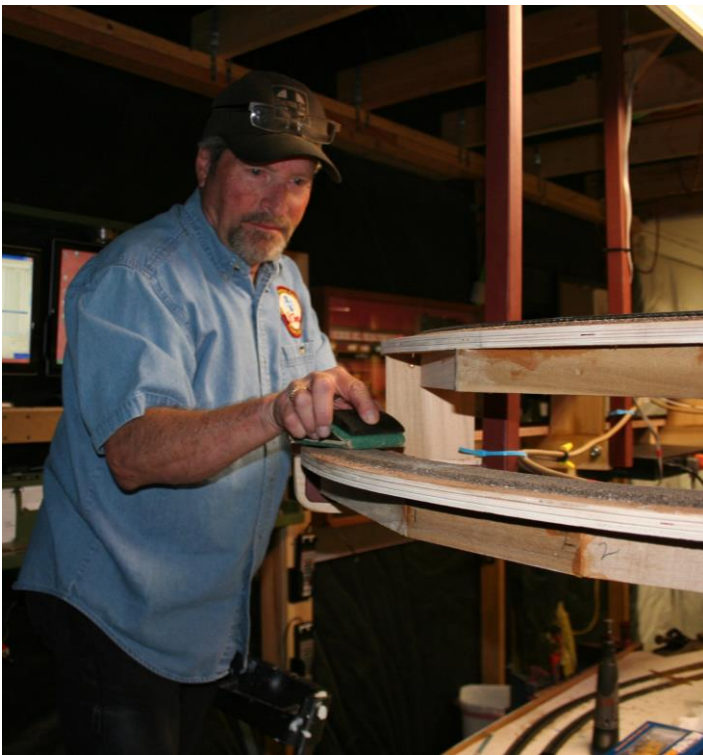
April 26, 2018: Left: Bruce is sanding the cork roadbed on the turn-around loop for the upper level off the end of the upper staging yard. Right: Kenneth is chasing control wiring for switches in the chase behind Texico and Canadian.
