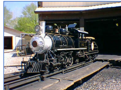
Locomotive 102 was built by Ted Young of Peoria IL. in 1983. The engine is a model of the Colorado Springs & Cripple Creek Railroad's full-sized 2-6-2 "Prairie" engines. Wabash, Frisco and Pacific Railroad photo
