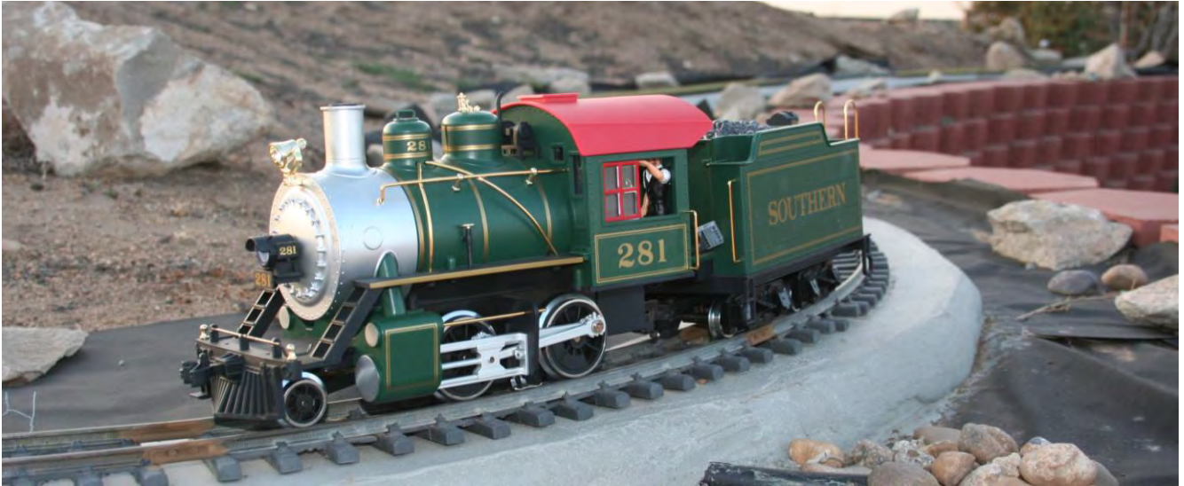
March 20: This is one of the first locomotives which is being equipped for battery-powered operation with radio control for use in the garden.
