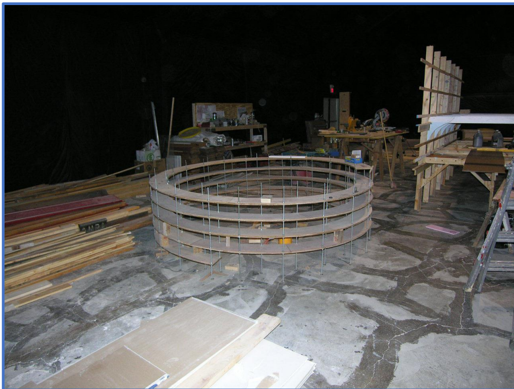
Top. A key component of the layout is connecting the lower to the upper level. Tracy Ball built an innovative double-tracked helix with threaded rod and nuts to adjust the rise of the sub-roadbed to a comfortable 1.3% grade. Bottom. A bit further down the road, is a photo of the helix in place.
