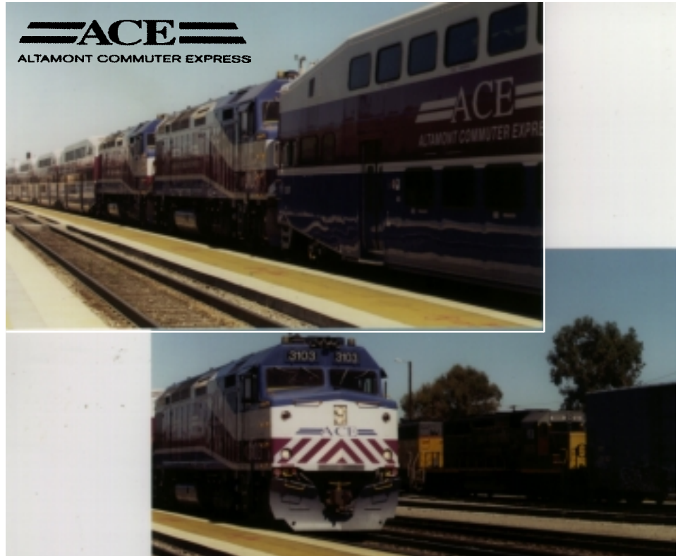
ACE SPECIAL ARRIVES FOR JAZZ FESTIVAL — With F40PH-3C No. 3103 on the point (lower right), the Altamont Commuter Express (ACE) train bound for the San Jose Jazz Festival on Saturday, 7 August, arrives in Santa Clara with a trailing "double consist" passenger train. The "mid-train helpers," a pair of F40PH-3Cs separate what are actually two trains. After dropping some passengers at the Great America stop for a day at the amusement park, the doubled train arrived in San Jose around 11:00 a.m. In the evening, these trains were split to enable departures at 6:00 p.m. and 8:00 p.m. This is the second year ACE has operated special trains from the Central Valley (Lathrop/Manteca) to San Jose for the Jazz Festival.
