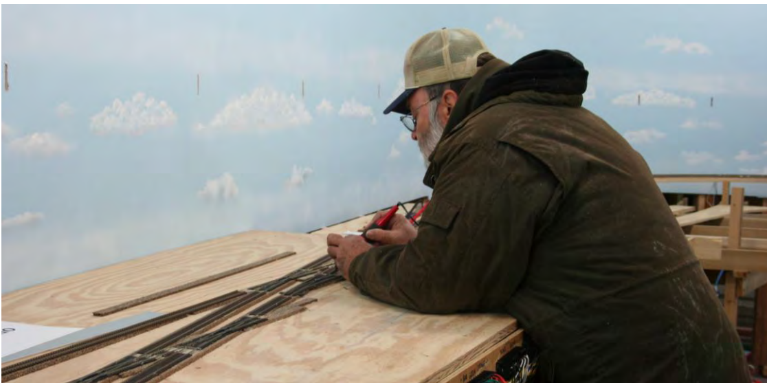
Jerry Michels soldering a drop on the frog of a turn-out in the East Tower area on November 23. It was cold inside the Train Room that day due to extremely cold temperature outside with strong North winds.
