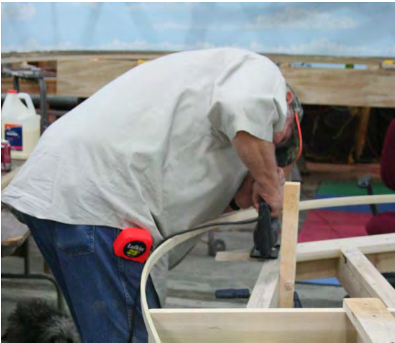
Virgil Doyle trimming-off the end of the top piece on a custom-built segment of L-girder.
