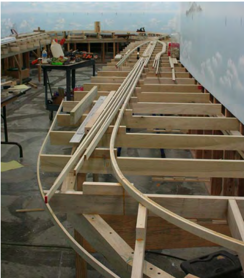
Spline sub-roadbed extending down the length of Kingsmill encompassing two main lines and sidings on both the North and South sides of the main lines. The core of the spline for the North main is wrapping the end of the peninsula extending East from Kingsmill toward Pampa in this photo.
