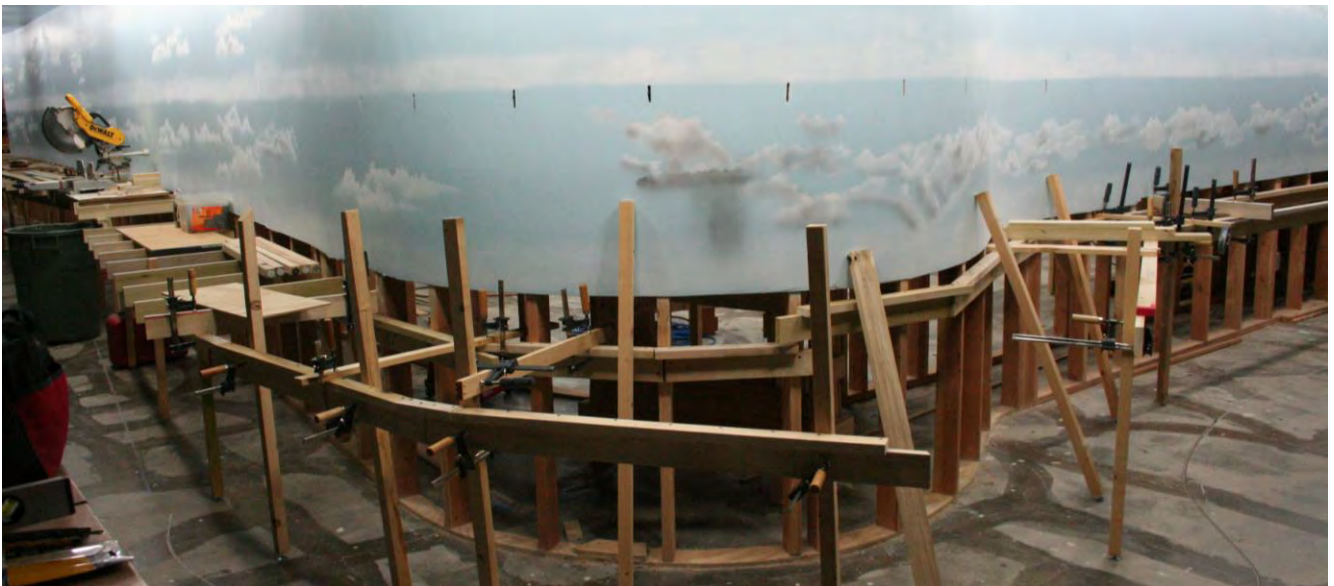
L-girder around the Northwest corner of the layout as it stood at the end of the work day on 3/23. The lowered L-girder in this area is to accommodate modeling of the Red Deer Creek area between Canadian and Miami.
