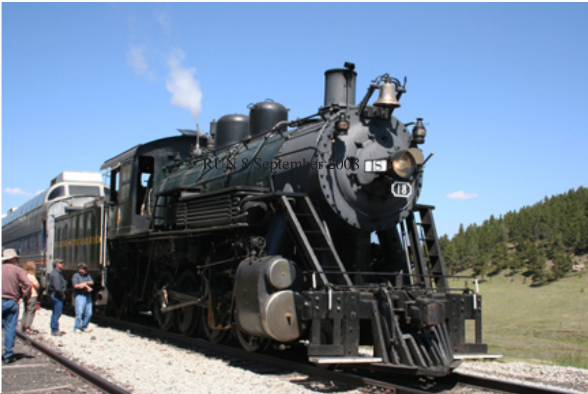
Rio Grande Scenic Railway # 18, a 2-8-0 of unknown heritage. Not a smooth rider.
